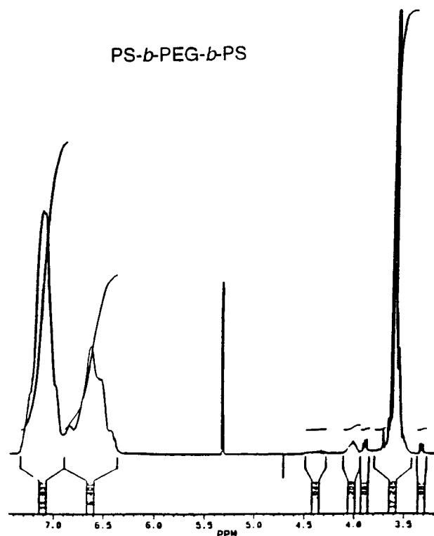
Figure 2. ^1\text{H} NMR spectrum of triblockcopolymer 2 in \text{CD}_2\text{Cl}_2 .
